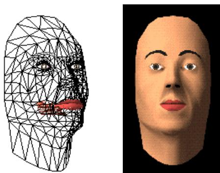
**Figure 5.11:** The figure shows a wire mesh model of a human face and the synthetic face, based on the model, used in the audio-visual speech synthesis project conducted at the ICP institute at the University of Grenoble [URL26].
