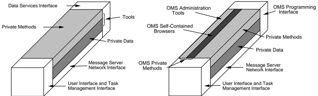
Figure 1: SEE-Reference Architecture / Data Integration by OMSs
