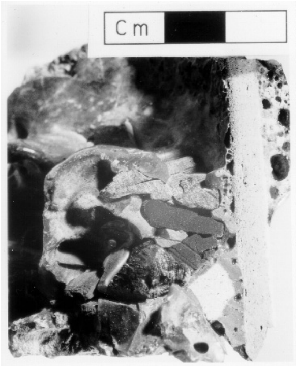
Fig. 11: Charcoal lumps (black) trapped in a glassy slag cake. The crucible wall (right) is overexposed to bring out the contrast between the dark slag and charcoal.
