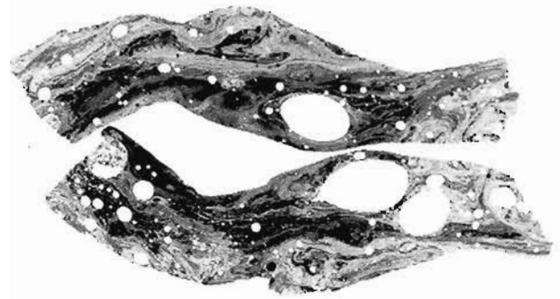
Fig. 3: Sample SS 89d: Droplet of ruby-red glassy slag. The streaks are caused by layers of copper and copper oxide inclusions. Width of the sample: 2.8 cm. Transmitting light.
