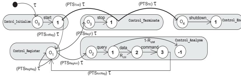
**Fig. 3.** Probabilistic LTS Synthesised for Component *Control*.
