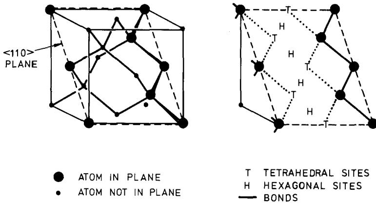
This energy surface is completely different from neutral hydrogen. The tetrahedral and hexagonal sites are high in energy with the minima along  $\langle 001 \rangle$  directions about 1.6 Å from a silicon atom. There is a saddle point between these sites along the back bond direction, but a direct route out of the  $\langle 110 \rangle$  plane between minima associated with different tetrahedral
