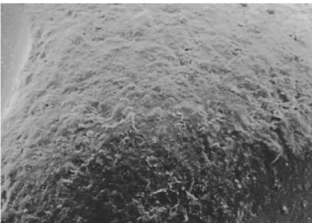
Figure 6 SEM micrograph of quartz sand grain exhibiting impact features caused during wind transportation. Scale bar 10 microns.
