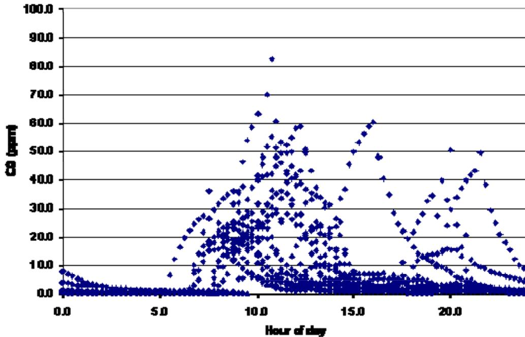
Figure 3: Time profile of CO concentrations for home shown in figure 2 (E11\_3LY\_274) all data for a period of about 10 days is presented by hour of the day, the highest peak occurs at hour 10.75 corresponding to 10:45am.
