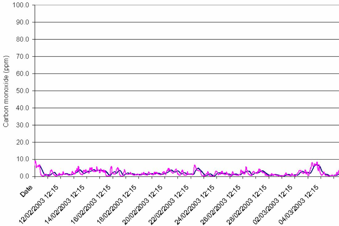
Figure 1: Carbon monoxide measurements from a typical home (E10\_5DS\_172), (the lighter line is the 15 minute average data, the darker smoothed line is the 8 hour moving average value) .
