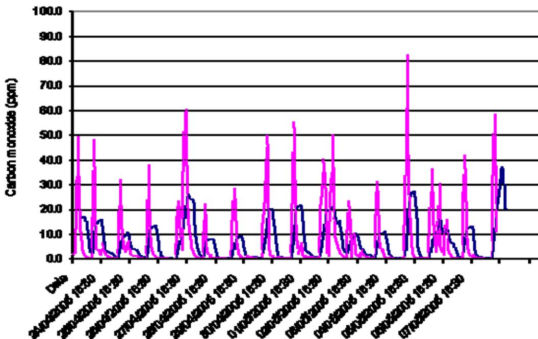
Figure 2: Carbon monoxide measurements from a home with a problem gas appliance (E11\_3LY\_274).
