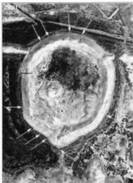
Figure 6 A satellite image of the earliest city at Merv, Erk Kala, showing the major rainwater erosion gullies (indicated by the arrows) and two deep channels in the entrance area shown (bottom centre of the city wall).
