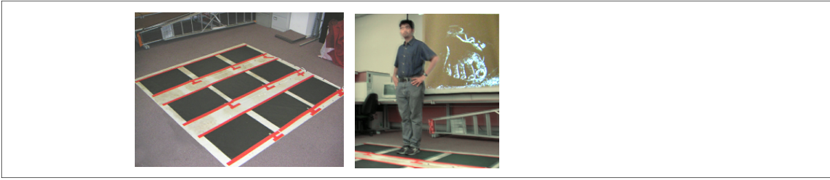
Fig. 6.1 Pressure mats and wires taped to the floor(left); test person on pressure mat (right).
