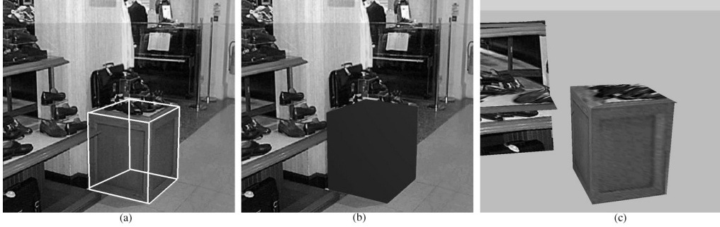
Fig. 1. (a) From within the environment, a user sketches over a box in a panoramic image. (b) The reconstructed object is left untextured. (c) If desired, the texture is grabbed from the background image.
