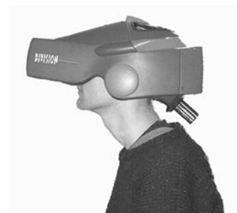
Fig. 3 A Virtual Reality Head Mounted Display [Source: http://www.vr.ucl.ac.uk/img/headset.jpg ]
