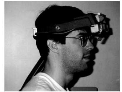
Fig. 5 See through head mounted display. [source: http://www.columbia.edu/cu/gsap/bt/RESEARCH/VR-CONST/vr-gear.jpg ]
