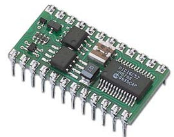
Fig. 42 Parallax BasicStamp2 as a stand alone product [source: ibid]
