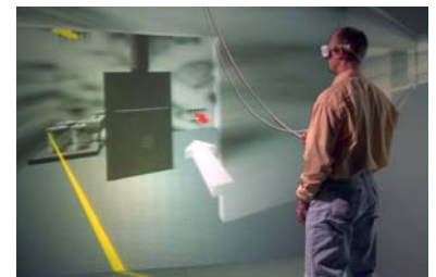
Fig. 4 A Virtual Reality CAVE (Cave Automatic Virtual Environment) [source: http://www_ivri.me.uic.edu/ivr1/contamination/vr.JPG ]
