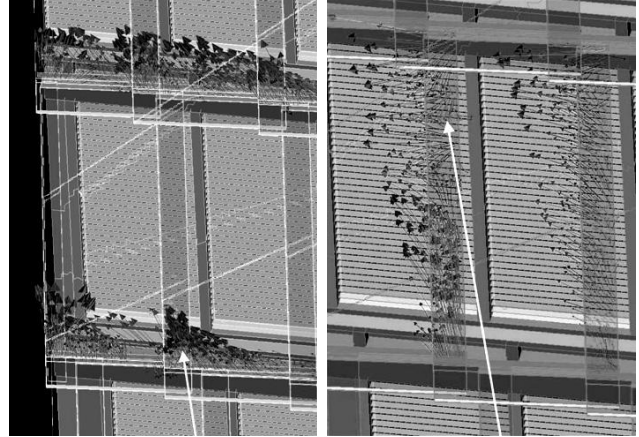
Figure 2. Exterior air enters the cavity through the opening at the bottom (left). Air rises as it heats up and is drawn to the left, exiting through the vertical slots between overlapping planes (right). Image: Kohn Pedersen Fox.
