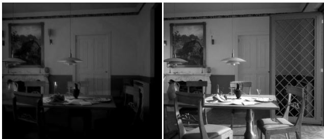
Figure 5. Multilight renders each light source separately so that they can be adjusted independently after rendering is complete. Different versions of the same scene can be produced without re-rendering. Image: Next Limit Technologies.
