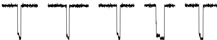
Figure 2.21. Examples of current modulations from Tyr 3 tagged oligonucleotides.
