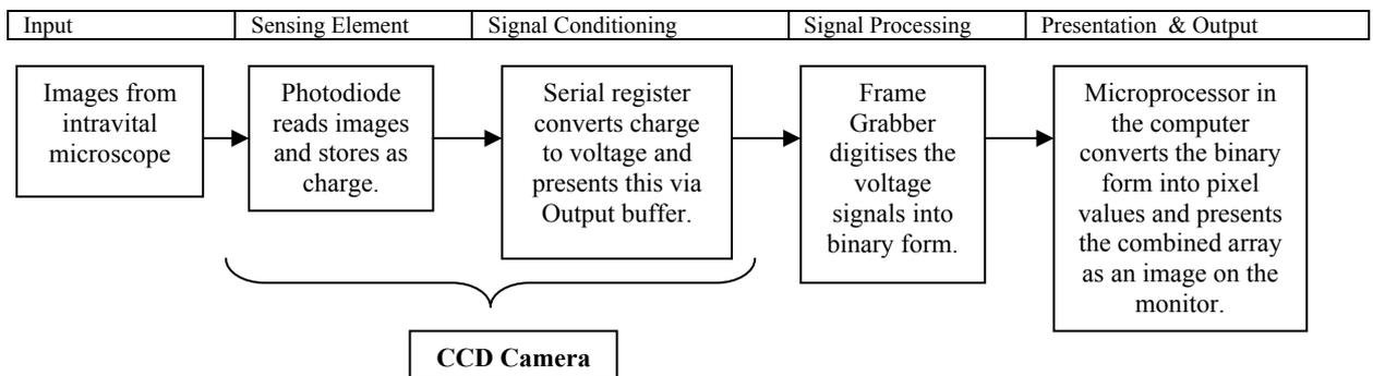
**Figure 1.4 Image recording system in the intravital microscope**
