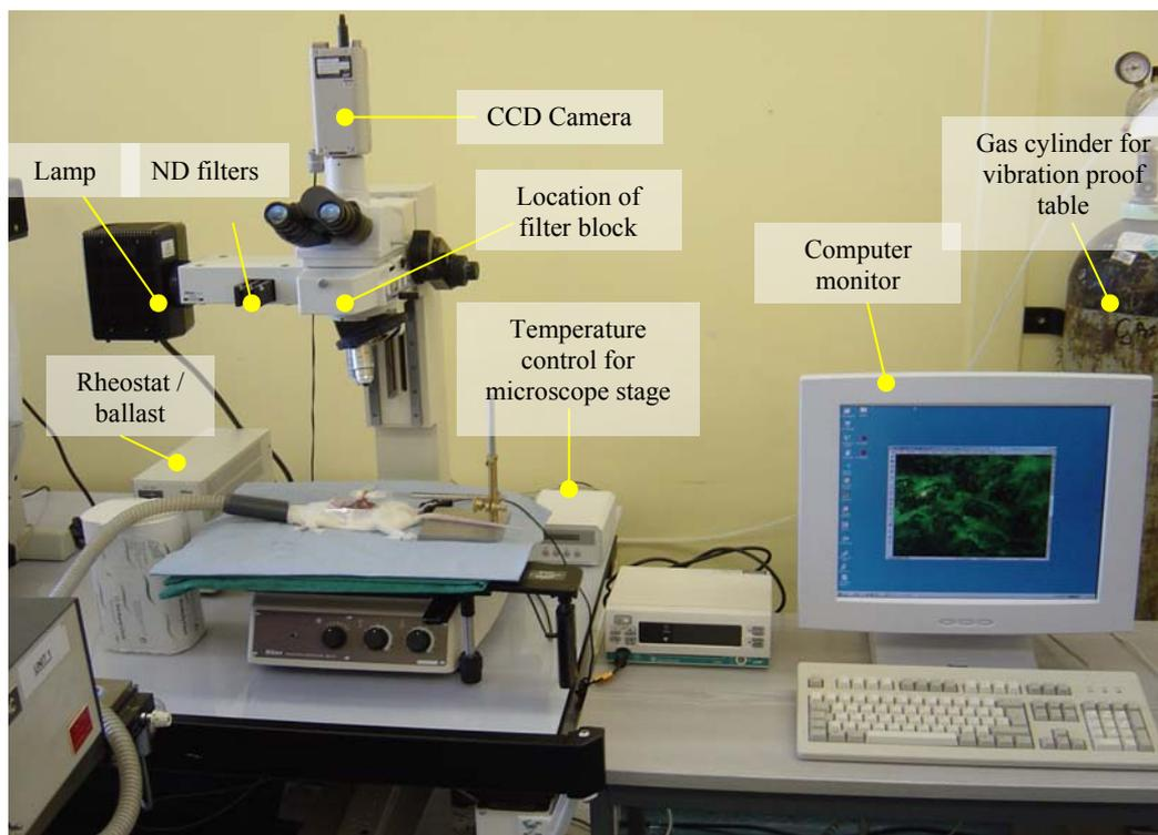
Figure 2.5 The complete intravital microscopy setup.
