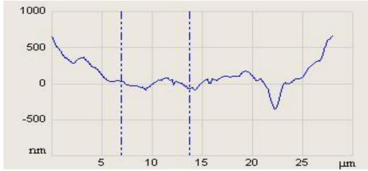
RMS polished end surface roughness: 26 nm to 192 nm.
