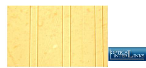
**Straight waveguides – Optical InterLinks**
