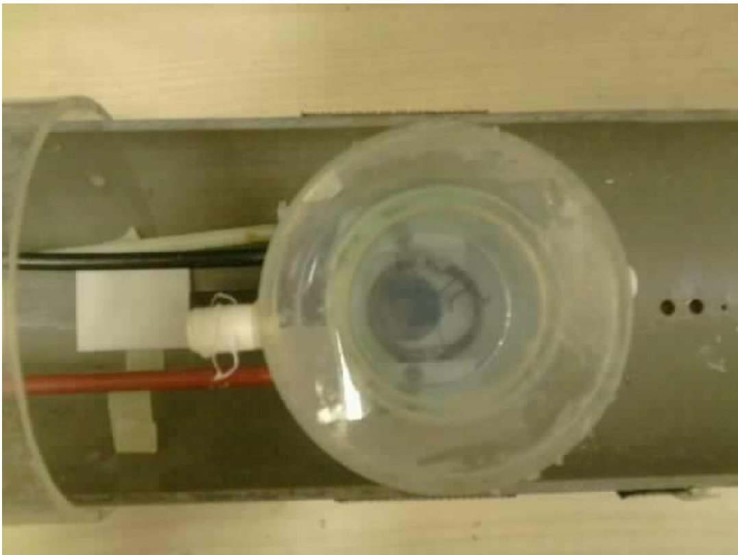
Figure 4.2b: Photographs showing the custom-made vessel for rat ^{31}\text{P} MRS experiments. Chilled fluid was circulated through the outer chamber with inlet and outlet ports for tubing connected to chiller machine. Additional tubing for oxygenation of PFC layer was attached to lid covering the vessel (not shown).
