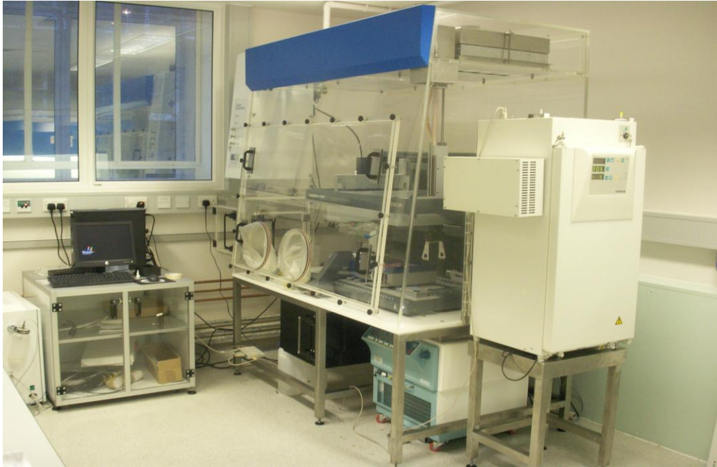
Figure 2.6 Automated system for the aseptic cell expansion culture of hMSC. The robotic platform that manipulates well-plate cultures is enclosed within a temperature and gas controlled biosafety cabinet. The system is equipped with a robotic incubator and a centrifuge, both of them with aseptic connections into the robotic platform.
