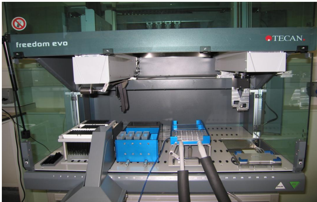
Figure 2.5 Tecan Automated Platform for the expansion of hMSC. The robotic arm on the right-hand-side transports the well-plates from the incubator to the platform. The liquid-handling arm on the left-hand-side can perform medium exchanges as well as trypsinisation operations by aspirating spent medium and dispensing new media or cell suspensions into the wells or well-plates.
