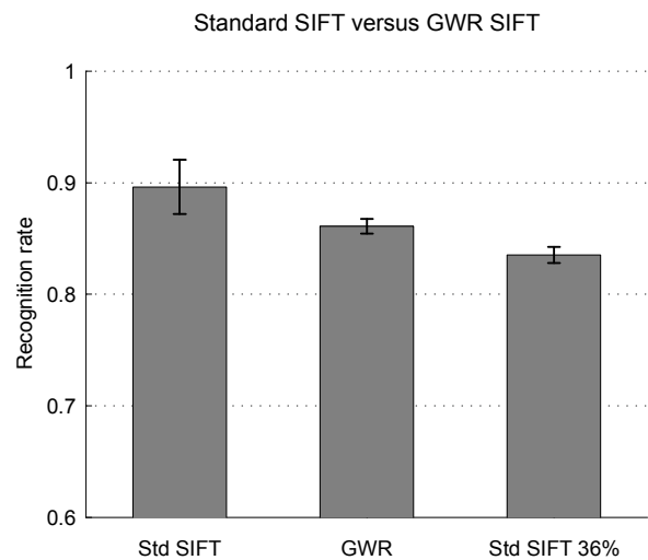
Fig. 4 The mean recognition rates for standard SIFT, the GWR-network and standard SIFT using 36% of the keypoint database. Standard SIFT uses on average 6429 keypoints. The GWR-network has on average 2396 keypoint clusters (37% of standard SIFT). For the GWR-network and SIFT using 36% keypoints, the data is acquired from 10 experimental runs. The error bars give the 95% confidence intervals.
