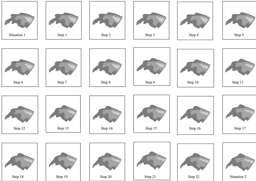
Figure 7. 22 Intermediate surfaces (microsteps) generated by blending the February, 1997 surface (Situation 1) into the September, 1997 (Situation 2) surface.
