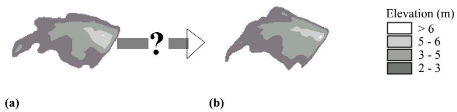
Figure 3. Digital elevation models of a sand spit at Scolt Head, Norfolk coast during (a) February, 1997 and (b) September, 1997.
