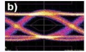
10 cm Waveguide with index matching fluid Jitter: 0.36 UI Relative Loss:: 4.5 dB
