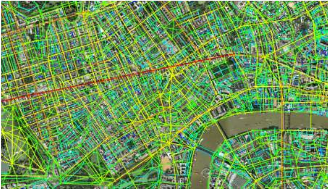
Figure 8 Part of central London, with an axial map superimposed coloured up for 'local integration', that is the closeness of each line to all others up to two turns away from each line
