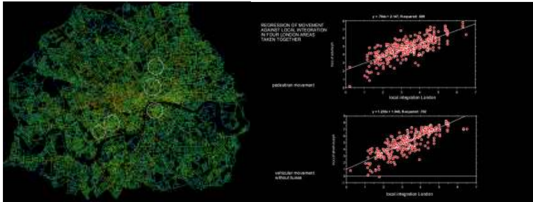
Figure 9 (left) An analysed axial maps of London within the North and South Circular Roads, coloured up for local integration with five selected areas within which observations of vehicular and pedestrians flows were made throughout the working day
