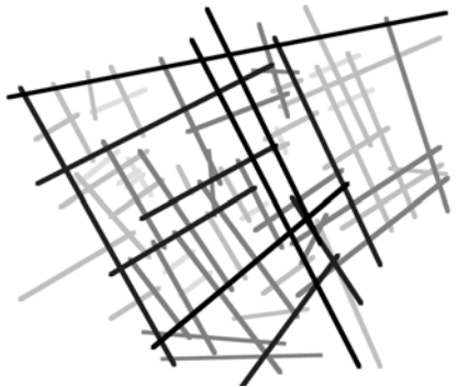
Figure 5c: Axial map processed to show calculation of radius n integration
