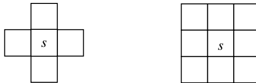
Figure 6.1: MRF neighbourhood systems for site s \in S . Left: first-order; Right: second-order.
