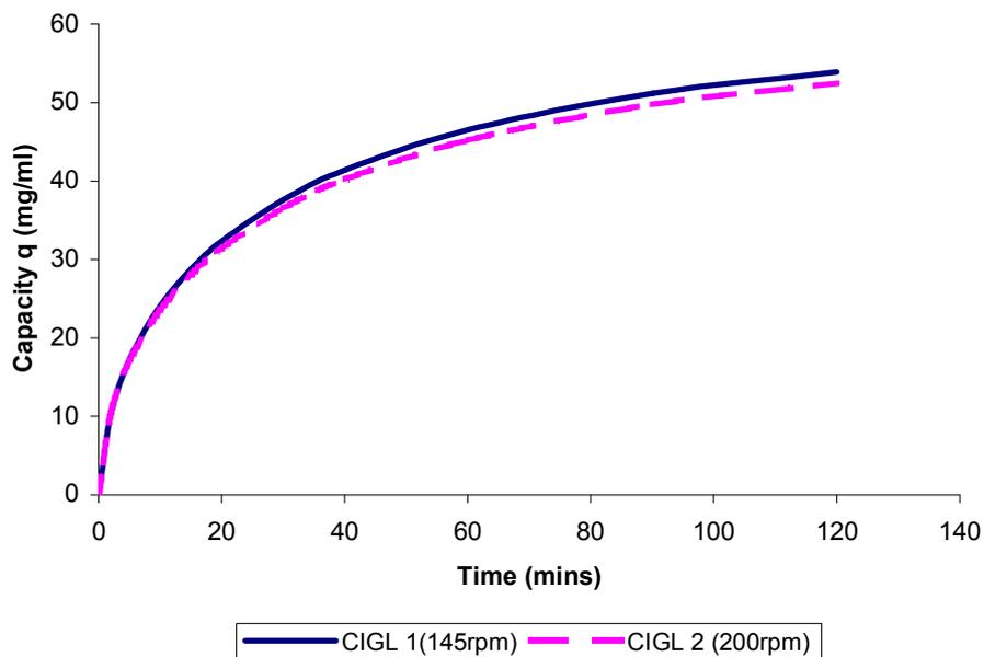
Fig 2.12 - Uptake kinetic curves for two samples of CIGL where the impeller speed of 145rpm and 200rpm was used to check mixing characterisation and reproducibility.
