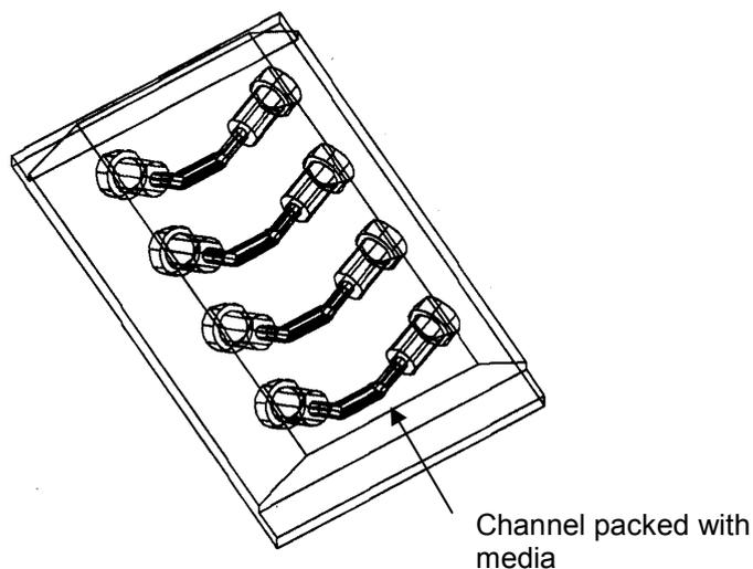
Fig 3.1- Flow cell with a channel of diameter 0.1cm and a length of 1cm was used to pack  $\sim 8\mu\text{l}$  of media, which could be placed under an inverted confocal microscope.
