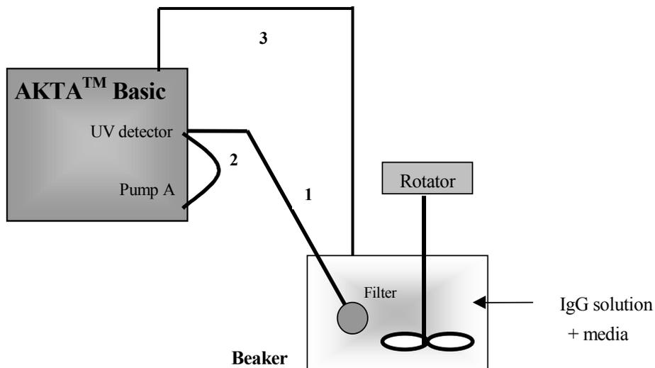
Tube 1 – Connected from filter to outlet of UV detector
