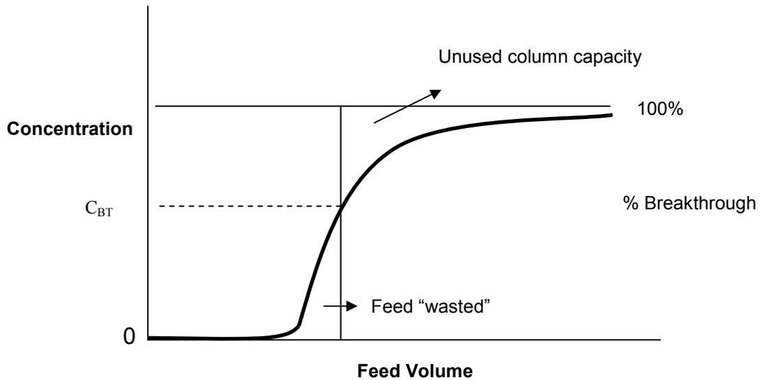
Fig 1.9 – Breakthrough curve
