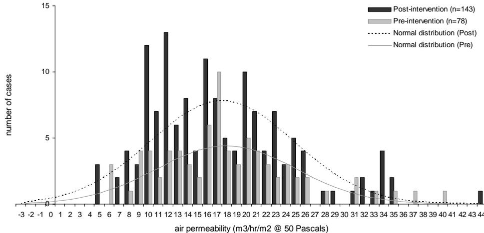
Figure 1: Air infiltration rate distribution for pre- and post-intervention WF dwellings
