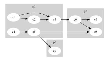
Fig. 1: Example of a Module Dependency Graph that is used to represent the modular structure of the systems under study. Nodes represent code elements and edges represent dependencies between elements. Clusters of nodes (grey regions) indicate high level modules.
