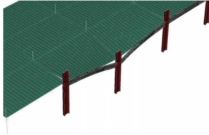
Fig. 6: Deformation state of the building after the column removal (1.60m displacement)
