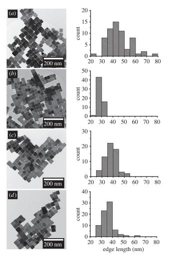
**Figure 5.** TEM images and corresponding size analysis of the extracted PbS nanocrystals formed within the S-polymer when using (a) 0.05 mmol, (b) 0.1 mmol, (c) 0.15 mmol and (d) 0.2 mmol of  $[Pb(S_2COOct)_2]$ .
