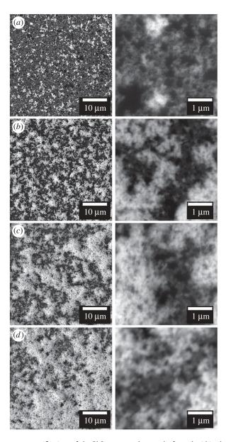
**Figure 4.** BSE-SEM images at two magnifications of the PbS nanocrystal networks formed within the S-polymer when using (a) 0.05 mmol, (b) 0.1 mmol, (c) 0.15 mmol and (d) 0.2 mmol of [Pb( $S_2$ COOct)<sub>2</sub>].
