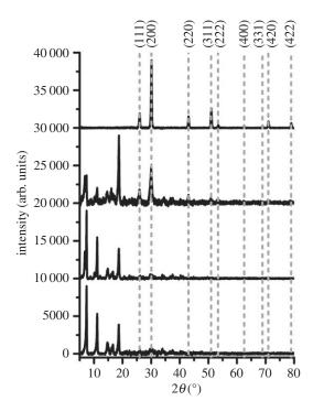
**Figure 3.** XRD patterns from the films of  $[Pb(S_2COOct)_2]$  decomposed within the S-polymer (from bottom to top): unreacted control, 50°C, 100°C and 150°C. Dashed lines represent the XRD pattern of PbS (galena), ICSD: 00-005-0592.
