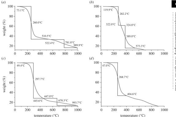
Figure 1. TGA profiles of: (a) pure poly(sulfur-co-1,3-diisopropenylbenzene) (1), (b) pure poly(sulfur-co-bisphenol A dimethacrylate) (2), (c) poly(sulfur-co-bisphenol A dimethacrylate-co-1,3-diisopropenylbenzene), higher ratio of 1,3-diisopropenylbenzene (3) and (d) poly(sulfur-co-bisphenol A dimethacrylate-co-1,3-diisopropenylbenzene), higher ratio of bisphenol A dimethacrylate (4).
