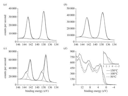
**Figure 2.** Pb 4f high-resolution XPS spectra are shown for films produced when decomposing  $[Pb(S_2COOct)_2]$  at: (a) 50°C, (b) 100°C and (c) 150°C. XPS valence spectra (d) showing the variation in the position of the Fermi level with heating temperature.
