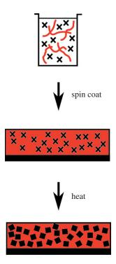
**Scheme 1.** The processing of precursor and polymer to form PbS nanocrystals within the sulfur polymer.
