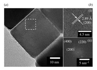
**Figure 6.** (a) HRTEM image of a PbS nanocrystal extracted from the film using 0.2 mmol of [Pb( $S_2$ COOct)<sub>2</sub>]. (b(i)) Expanded image from the white box region showing the  $\langle 200 \rangle$  plane of PbS (qalena) and (b(ii)) fast Fourier transform of the selected region.
