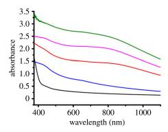
**Figure 7.** UV/visible spectra of films containing different concentrations of  $[Pb(S_2COOct)_2]$ : 0.1 mmol in polymer (4) prior to decomposition (black), and after heating 0.05 mmol (blue), 0.1 mmol (red), 0.15 mmol (pink) and 0.2 mmol (green).
