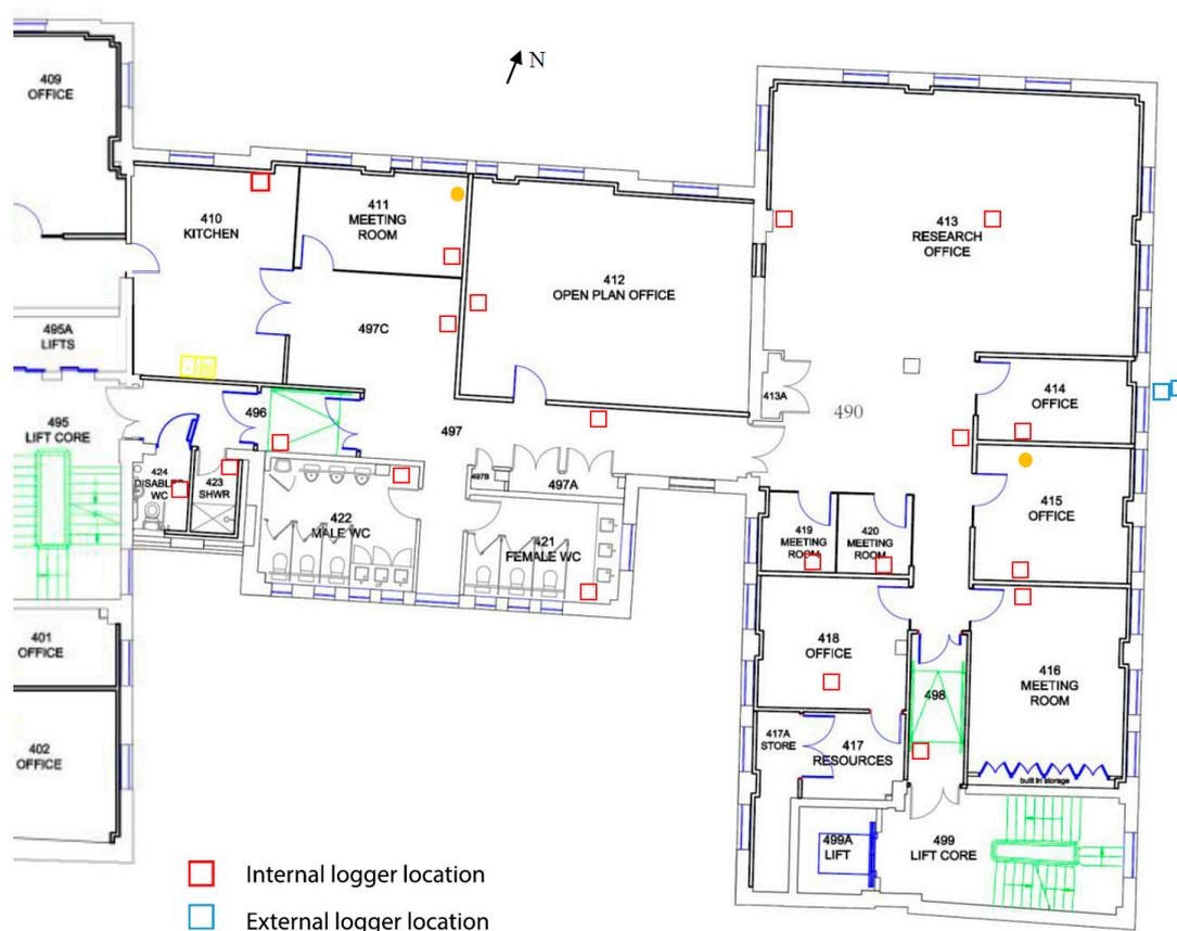
**Figure 3.** Central House 4th floor, with logger locations.
