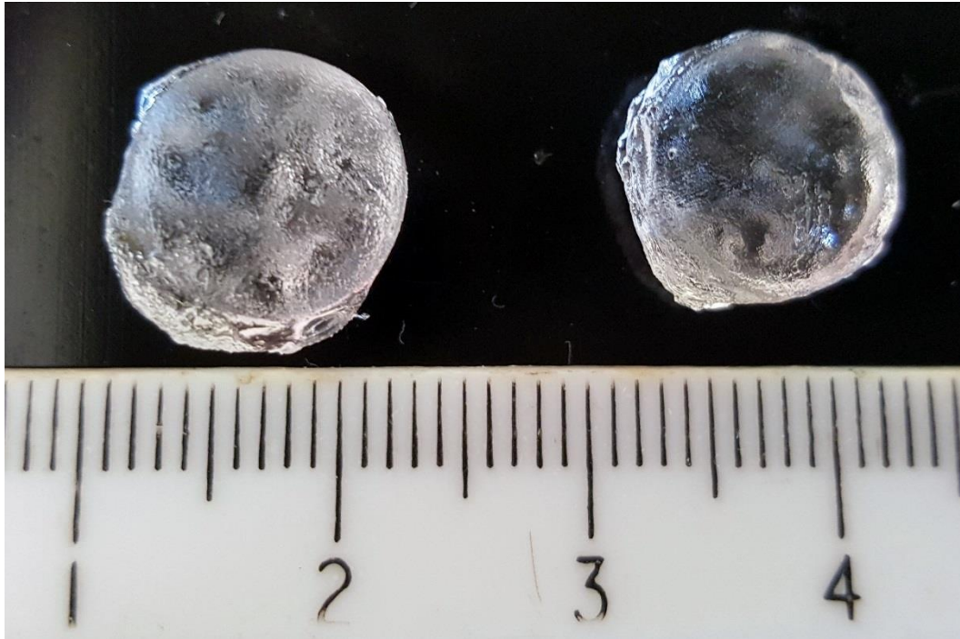
Figure 1. Hydrogels printed with DPPO as the photoinitiator, showing poor repeatability of size and shape. The scale is shown in cm.
