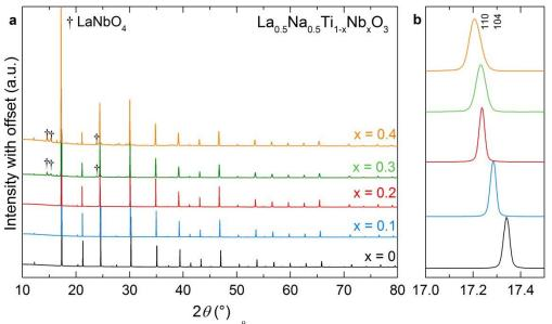
**Fig. S4.** SXRD ( $\lambda = 0.826119$  Å) data measured on samples in the composition range La<sub>0.5</sub>Na<sub>0.5</sub>Ti<sub>1-x</sub>Nb<sub>x</sub>O<sub>3</sub>. Pure samples were obtained up to x = 0.2, above which small amounts of LaNbO<sub>4</sub> were observed. Composition dependence of the position of the 110 and 104 reflections is highlighted in b).
