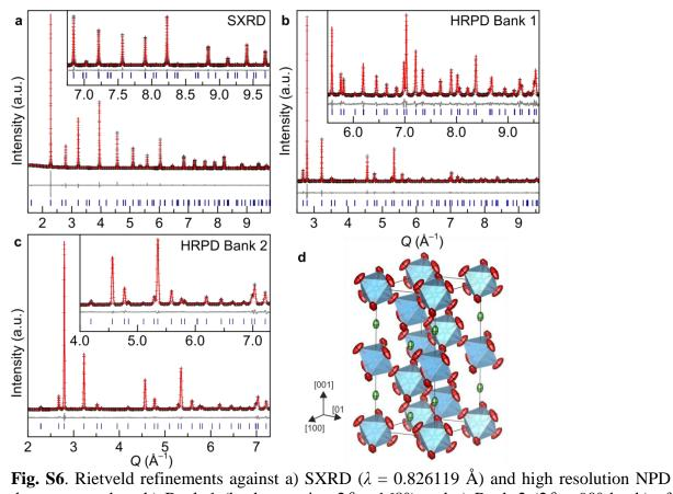
**Fig. S6.** Rietveld refinements against a) SXRD ( $\lambda = 0.826119$  Å) and high resolution NPD data measured on b) Bank 1 (backscattering  $2\theta = 168^{\circ}$ ) and c) Bank 2 ( $2\theta = 90^{\circ}$  bank) of HRPD at room temperature for La<sub>0.5</sub>Na<sub>0.5</sub>Ti<sub>0.8</sub>Nb<sub>0.2</sub>O<sub>3</sub>.
