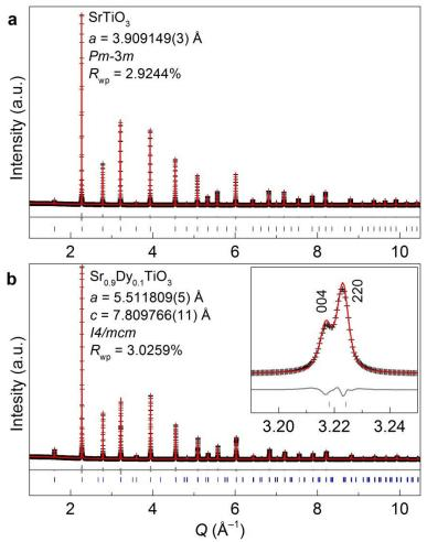
**Fig. S13**. Rietveld refinements against SXRD ( $\lambda = 0.826119$  Å) data measured from a) SrTiO<sub>3</sub> and b) Sr<sub>0.9</sub>Dy<sub>0.1</sub>TiO<sub>3</sub>. The inset in b) shows the splitting of the 004 and 220 reflections in tetragonal Sr<sub>0.9</sub>Dy<sub>0.1</sub>TiO<sub>3</sub>.
