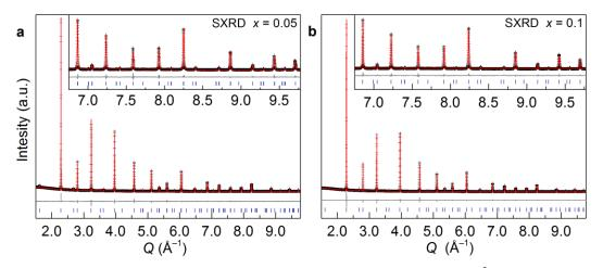
**Fig. S7**. Rietveld refinements made against SXRD ( $\lambda = 0.826119$  Å) data for the a) x = 0.05 and b) x = 0.1 doped materials in the La<sub>0.5</sub>Na<sub>0.5</sub>Ti<sub>1-x</sub>Nb<sub>x</sub>O<sub>3</sub> solid solution.
