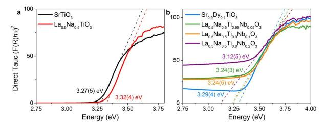
**Figure S8**. Tauc plots of direct band gaps calculated using the Kubelka-Munk function F(R) obtained from diffuse reflectance measurements for a) SrTiO<sub>3</sub> and La<sub>0.5</sub>Na<sub>0.5</sub>TiO<sub>3</sub>, and b) Sr<sub>0.9</sub>Dy<sub>0.1</sub>TiO<sub>3</sub>, and La<sub>0.5</sub>Na<sub>0.5</sub>Ti<sub>1-x</sub>Nb<sub>x</sub>O<sub>3</sub> (where x = 0.05, 0.1 and 0.2).
