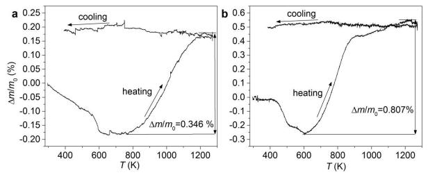
**Fig. S14.** Relative weight change for a)  $Sr_{0.9}Dy_{0.1}TiO_3$  and b)  $La_{0.5}Na_{0.5}Ti_{0.8}Nb_{0.2}O_3$  as a result of oxidation from heating up to 1273 K under air. The data show oxidation to take place at approximately 750 K and 600 K for  $Sr_{0.9}Dy_{0.1}TiO_3$  and  $La_{0.5}Na_{0.5}Ti_{0.8}Nb_{0.2}O_3$ , respectively. The materials were white in colour after cooling to room temperature.
