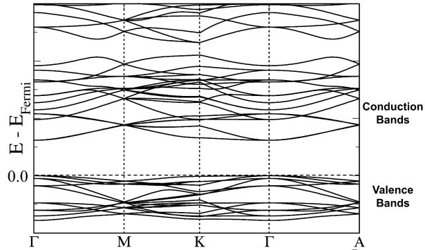
**Fig. S17**. The full band structure of cubic STO (in a rhombohedral cell with  $R\overline{3}c$  space group symmetry and with zero tilting). All the bands have been aligned to the Fermi level.
