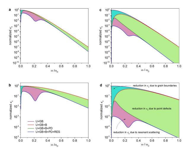
**Fig. S2**. Calculated spectral thermal conductivity  $\kappa_S$  for Sr<sub>0.9</sub>Dy<sub>0.1</sub>TiO<sub>3- $\delta$ </sub> at a) 25K and b) 80K and La<sub>0.5</sub>Na<sub>0.5</sub>TiO<sub>3</sub> at c) 25K and d) 80K, illustrating the contribution of different scattering mechanisms in decreasing  $\kappa_S$  (blue: grain boundaries, green: point defects and purple: resonant scattering).
