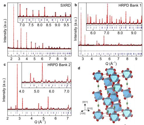
**Fig. S1**. Rietveld refinements against a) SXRD ( $\lambda = 0.826119$  Å) and high resolution NPD data measured on b) Bank 1 (backscattering  $2\theta = 168^{\circ}$ ) and c) Bank 2 ( $2\theta = 90^{\circ}$  bank) of HRPD at room temperature for La<sub>0.5</sub>Na<sub>0.5</sub>TiO<sub>3</sub>.
