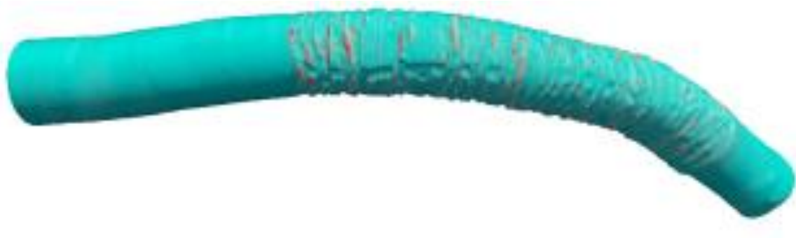
Figure 4. Recirculation zones (red) were quantified based on the ESS and the centerline direction (proximal → distal). The red areas in the luminal surface are where the vectors of the ESS are pointing opposite (more than 90-degrees away from) the proximal-to-distal direction along the centerline.
