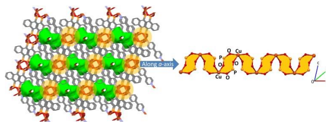
Figure 1. The 3D structure of 1 , showing the voids highlighted in green within the framework and 1D SBU composed of edge sharing Cu-O-P-O-Cu-O-P-O rings.
