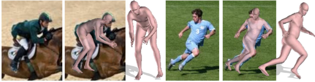
Figure 3.6: 3D pose and shape estimation results on two example images from the Leeds Sports Pose Dataset [61]. From left to right: the input image, fitted model and the 3D shape rendered from a new viewpoint. Figure from [11].
