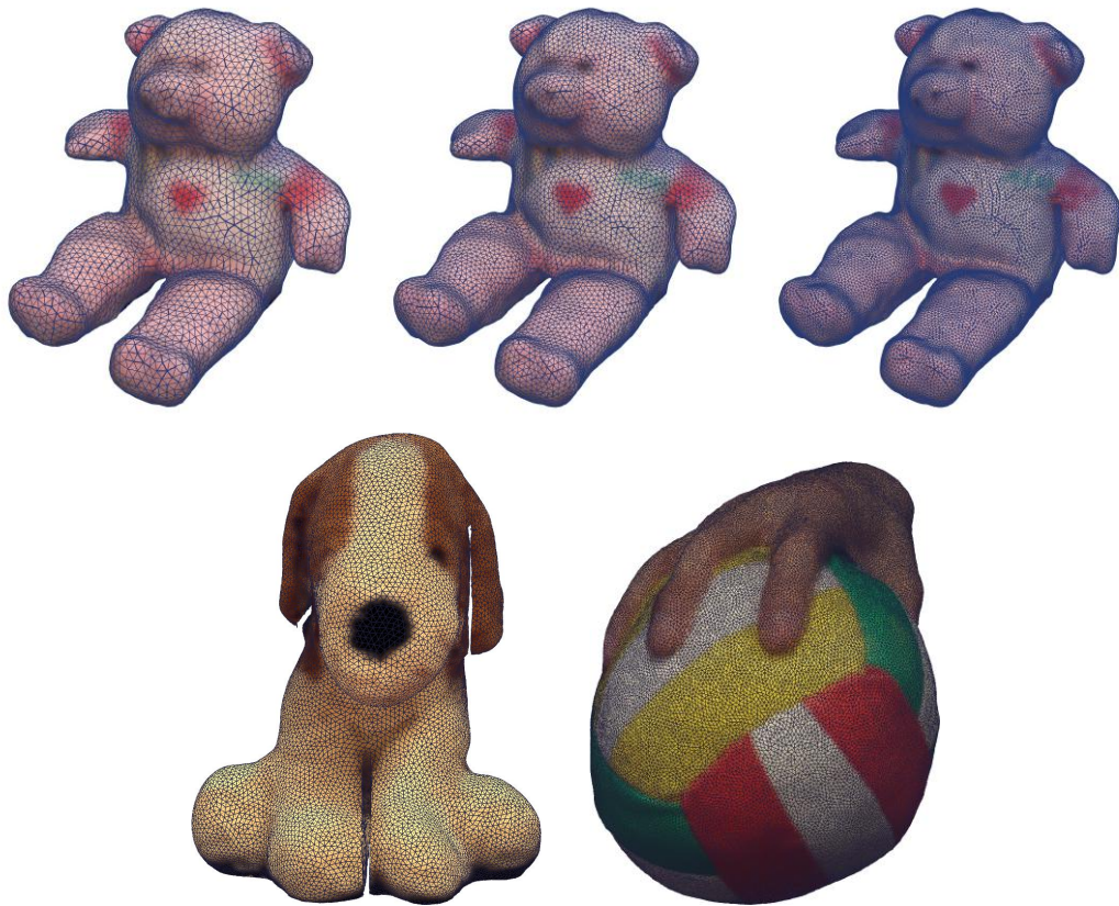
Figure 5.2: An example of our multi-scale template meshes generated by iterative mesh down-sampling and refinement. Top: From left to right the meshes contain approximately 5, 10, and 25 thousand vertices respectively. Bottom: The highest levels of the templates for the dog and ball sequences.
