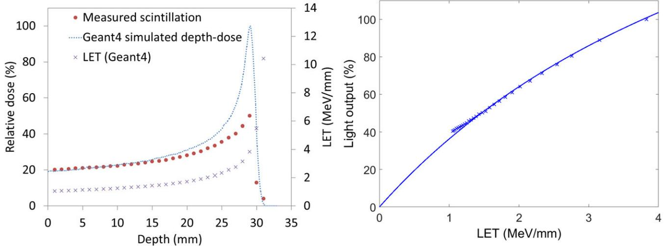
**FIG. 5.** (a) LET values simulated by Geant4, depth dose profile simulated in Geant4, and the measured scintillation light distribution as a function of depth for a 60 MeV proton beam in a BC-408 scintillator (b) The measured scintillation light vs simulated LET for the 60 MeV proton beam (note that the highest LET points do not contribute to light output as they occur beyond the Bragg peak).
