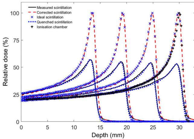
**FIG. 6.** Percentage depth dose curves at 38.94, 46.77, 53.86, and 60.00 MeV, showing (a) the simulated depth dose (blue crosses); (b) the depth dose directly measured by the camera (solid black line); (c) the simulated quenched light output (blue bars); and (d) the measured light output after correction for quenching (red dashes).
