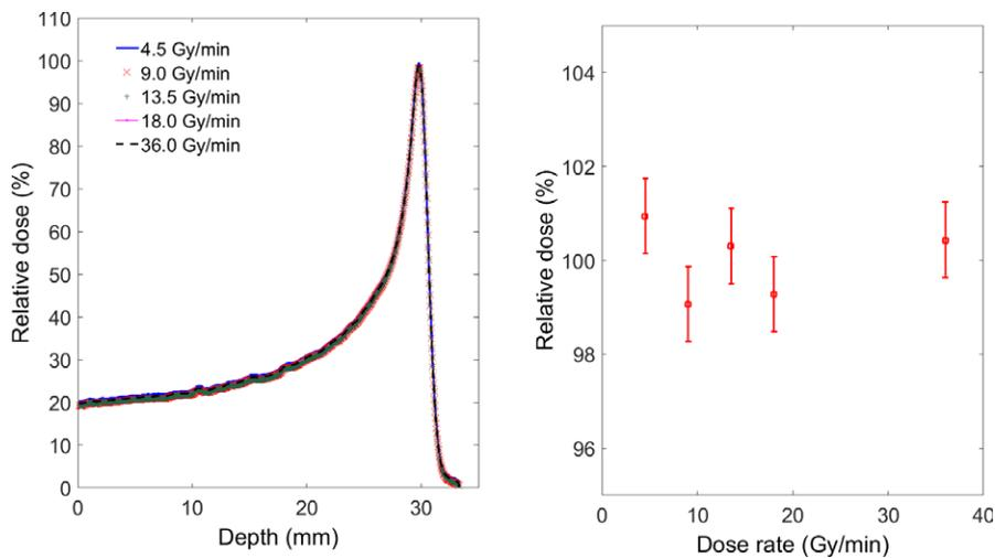
**FIG. 8.** The response of the scintillation detector system after delivering 4.5 Gy at different dose-rates for a 60 MeV proton beam. Vertical bars on the right hand graph give the measurements error.
