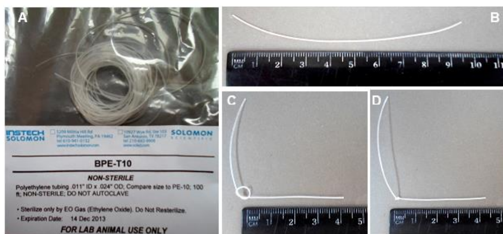
Fig. 1. Photographs of PE-10 tubing used in the study (A) and a fabricated catheter of 10-cm long cut (B) with a knot made approximately at the middle (C), tightened then out (D).
