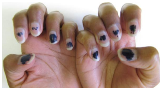
Fig 1. Photograph shows that the residence of the same nail varnish film (blue-coloured for visibility in this experiment) is highly variable on the different fingernails. Consequently, to compare nail lacquers, every nail lacquer should be applied to all the fingernails (rather than apply a different lacquer to a different nail).
