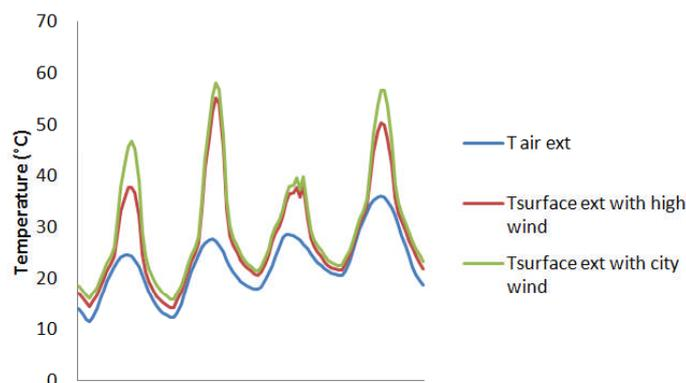
Figure 6 : Four days of simulation in July with EnergyPlus - Surface temperatures with different wind speed on top floor of stand-alone building
