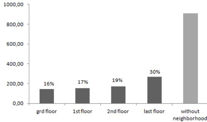
Figure 3 : Access to solar radiation in kWh/m<sup>2</sup> per year and percentage of solar radiation available at this solar orientation for each façade with neighbourhood, EnergyPlus calculations.
