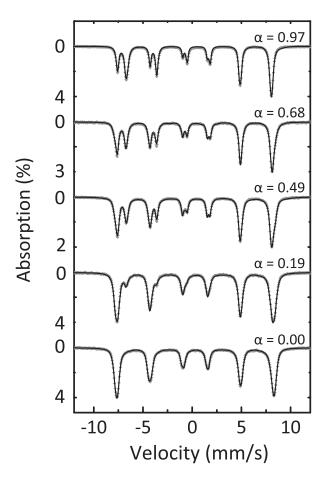
**Figure 2.** <sup>57</sup>Fe Mössbauer spectra, recorded at room temperature  $(T=295\pm5\,\mathrm{K})$ , of polycrystalline samples of magnetite, Fe<sub>3</sub>O<sub>4</sub> (sample DTU100,  $\alpha=0.97\pm0.02$ , top) and maghemite,  $\gamma$ -Fe<sub>2</sub>O<sub>3</sub> (sample DTU0,  $\alpha=0.00\pm0.01$ , bottom), and of mixtures of the two phases. The solid lines represent the best-fit results using the model-independent curve-fitting procedure described in section 3.
