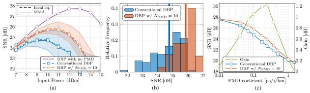
Fig. 3. (a) Average SNR versus input power. The shaded areas represent the standard deviation. (b) Histogram of the SNRs obtained by DBP and the proposed modification. The vertical thin bars represent the mean values. (c) Average optimum SNR and SNR gain versus the fiber PMD parameter obtained at the optimum input power for each scenario.
