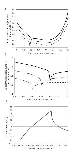
Figure 7: The effect of shear-thinning when  $\beta=Re=0$ . (a) Plot of the critical Weissenberg number  $W_{\rm crit}$  against relaxation time power-law n, for three different values of the shear-stress power law m. Solid line: m=0.20 (identical to figure 5 of [2]; dotted line: m=0.19; dashed line: m=0.18. (b) Small region of plot (a). (c) Dependence of the growth rate on m for specific values of the other parameters: n=0.4, W=2, k=3, Re=0,  $\beta=0$ .
