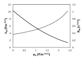
Figure 1: Plot of the required behaviour of the parameters  $G_M$  (solid line) and  $K_M$  (dashed line) as the solvent coefficient  $\mu_0$  varies, in order to correctly replicate the experimental data from [1]. Curves specified by equation (16).
