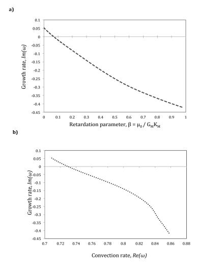
Figure 2: Variation of the instability with the retardation parameter  $\beta$  at  $m=0.2,\ n=0.4,\ W=2,\ Re=0$  and k=3. (a) Plot of growth rate  $\Im(\omega)$  against  $\beta$ . (b) Behaviour of the eigenvalue  $\omega$  in the complex plane.
