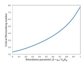
Figure 6: Plot of the critical Weissenberg number against the retardation parameter  $\beta$  for an exemplar fluid defined by  $m=0.2,\,n=0.4.$
