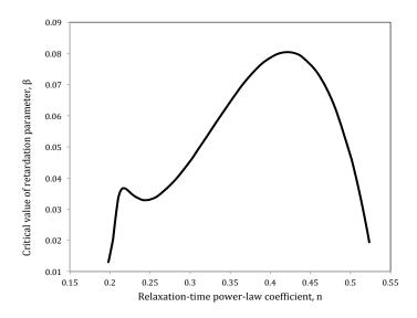
Figure 4: Critical retardation parameter value  $\beta$  plotted against relaxation time power-law n; the other parameters are fixed as  $m=0.2,\,Re=0,\,W=2.$
