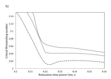
Figure 5: Critical Weissenberg number plotted against the relaxation time power-law, n, for different values of the retardation parameter  $\beta$ , in the absence of inertia (Re=0). We have fixed m=0.2. (a) Increasing from bottom:  $\beta=0,\,0.01,\,0.04,\,0.046,\,0.05,\,0.1$ ; (b) the disappearance of the local minimum near n=0.2: (from bottom)  $\beta=0.04,\,0.046,\,0.05$ .
