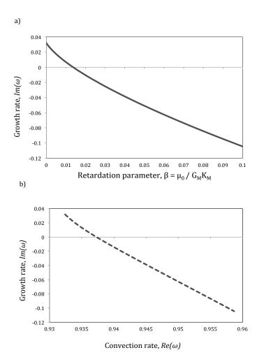
Figure 3: Variation of the instability with the retardation parameter  $\beta$  for a fluid with constant shear modulus constant: m=n=0.2, W=2, k=3 and Re=0. (a) Plot of growth rate  $\Im(\omega)$  against  $\beta$ . (b) Behaviour of the eigenvalue  $\omega$  in the complex plane.
