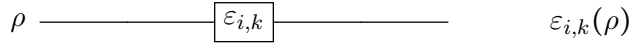
Figure 2.5: Effective channel implemented by the building block. The building block effectively implements a quantum channel \varepsilon_{i,k} on the input state \rho where i refers the measurement bases and k the measurement outcome.
