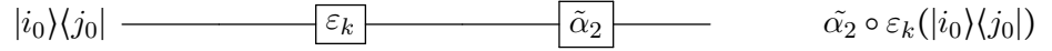
Figure 2.16: Effective resulting channel: noisy resource. A noisy resource state effectively corresponds to the channel \varepsilon followed by \tilde{\alpha}_2 being applied to the input.
