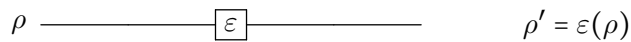
Figure 2.1: Single qubit quantum channel. The initial state \rho is mapped to a new state \rho' = \varepsilon(\rho) by the application of a quantum channel.
