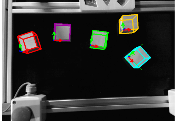
Figure 6. Initialisation of trackers for all blocks in the very first image. The wire frames illustrate the object CAD models. These are projected onto the image using initial poses supplied by the human operator.
