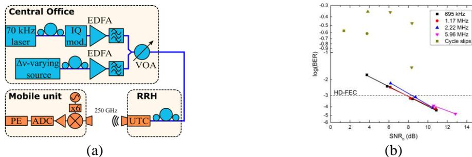
**Fig.1:** (a) Experimental setup and (b) receiver tolerance to THz signal linewidth. RRH: remote radio head; VOA: variable optical attenuator; UTC: uni-traveling-carrier photodiode; ADC: analog-to-digital converter.
