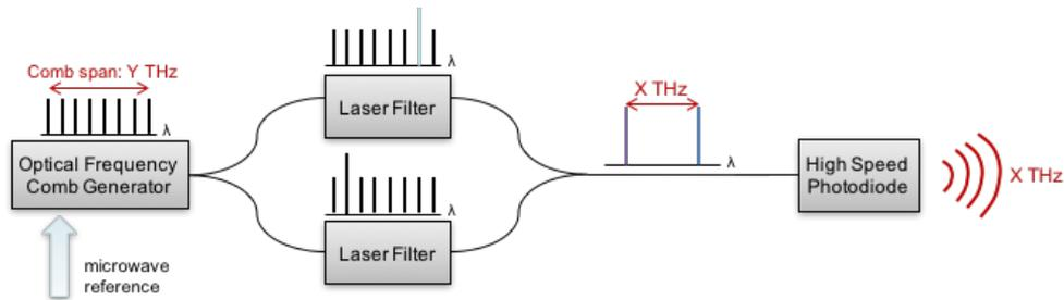
**Fig. 1: Schematic of a typical heterodyne THz source.**
