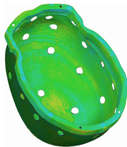
Figure 5. Deviation analysis comparing 3D scan of adult tank to target CAD model.
