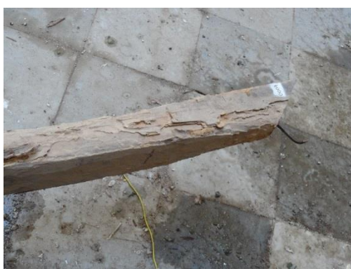
Figure 7.45 Yielding of the nail of a connection of the Cathedral of Ica (courtesy of Erika Vicente, PUCP)
