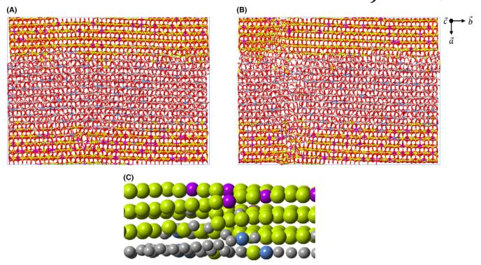
**FIGURE 4** A and B, Stick representations of two different sections of the GDC/YSZ bulk. C, ball representation of a screw dislocation observed in the GDC phase near the interface with YSZ, with the oxygen atoms omitted for clarity.  $Ce^{4+}$ : green,  $Gd^{3+}$ : magenta,  $O^{2-}$ : red,  $Y^{3+}$ : blue, and  $Zr^{4+}$ : gray. [Color figure can be viewed at wileyonlinelibrary.com]
