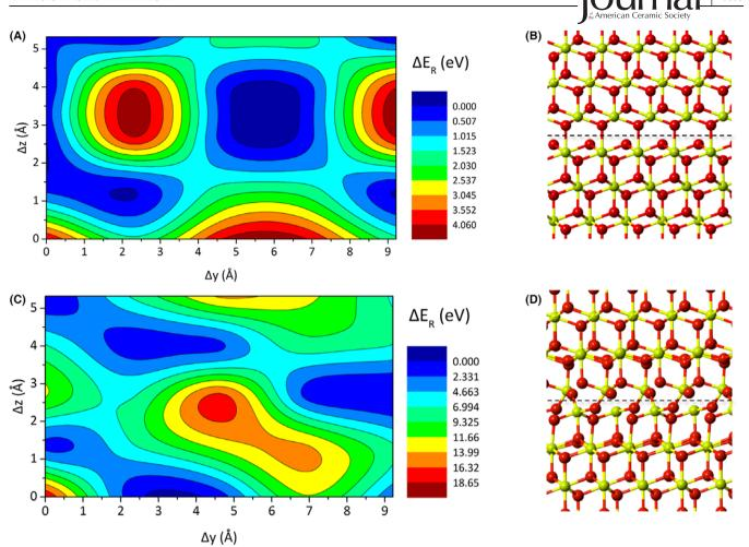
**FIGURE 2** IPES for (A) GB-O<sub>t</sub> and (C) GB-M<sub>t</sub>, and the corresponding ball and stick representations for (B) GB-O<sub>t</sub> and (D) GB-M<sub>t</sub> which is lower in energy [Color figure can be viewed at wileyonlinelibrary.com]
