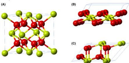
**FIGURE 1** Ball and stick representation of (A) fluorite-type unit cell; (B) oxygen termination of the (111) surface derived from a fluorite-like system; and (C) metal termination of the (111) surface derived from a fluorite-like system. Cations are represented in green, whereas oxygen atoms are represented in red. Atomic radii are chosen randomly to aid clarity [Color figure can be viewed at wileyonlinelibrary.com]
