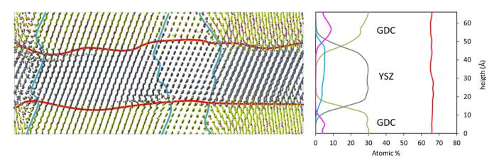
**FIGURE 5** (Left) Ball and stick representation of the GDC/YSZ model obtained after applying A&R strategy. Oxygen atoms are not represented for simplification. (Right) Concentration profile for the different atomic species.  $Ce^{4+}$ : green,  $Gd^{3+}$ : magenta,  $O^{2-}$ : red,  $Y^{3+}$ : blue, and  $Zr^{4+}$ : gray [Color figure can be viewed at wileyonlinelibrary.com]
