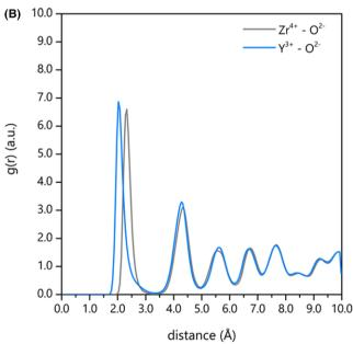
**FIGURE 6** Radial distribution functions, g(r), for the different cation-anion pairs at 10 K in (A) the gadolinium-doped ceria phase and (B) the yttria-stabilized zirconia phase [Color figure can be viewed at wileyonlinelibrary.com]
