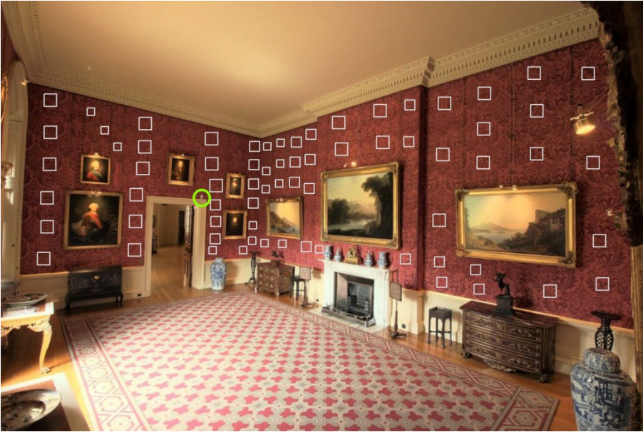
Figure 3. The distribution of reference patches on the wallpaper selected to permit interpolation of illuminance values derived from luminance values generated by HDR
